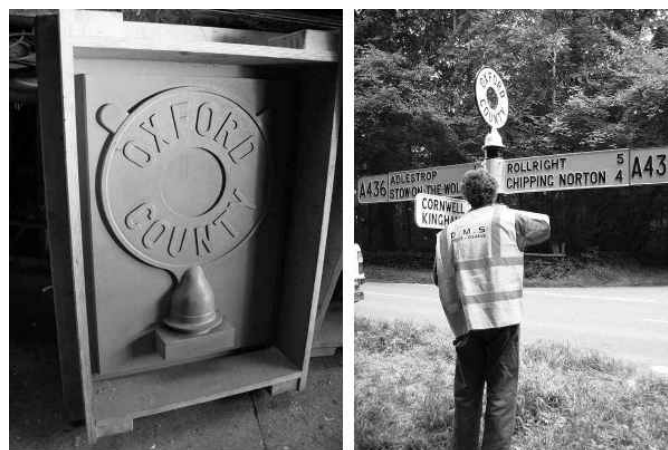
The 'OXFORD COUNTY' finial pattern, an essential item when casting new parts for the Oxon fingerposts. On the right is Mike Mulligan of DMS putting the finishing touches to the Cornwell post on the A436. [Photos - Mike Mulligan]
